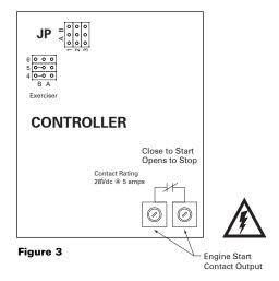
The engine-start terminals are clearly identified by a label on the microcontroller backplate. In the case of manual transfer switches, or in other applications not requiring the microprocessor, clearly marked terminal blocks are provided in the upper left corner of the control panel for the engine start control wires.
